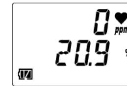
Upper row: [CO] (carbon monoxide) gas concentration display Middle row: [O2] (oxygen) gas concentration display
