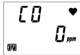
[CO] (carbon monoxide) gas concentration display
